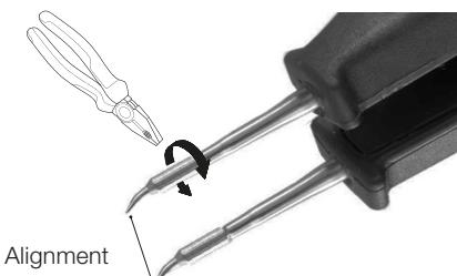
Align the tip of the cartridge. Use a flat pliers for a correct tip alignment.
