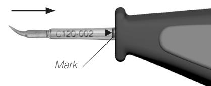
**Important:** Insert the cartridge as far as the mark for a correct connection.
