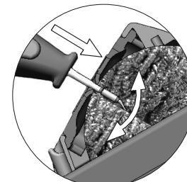
If the tip is very dirty, JBC recommends first cleaning it with the wiper to remove excess solder.
