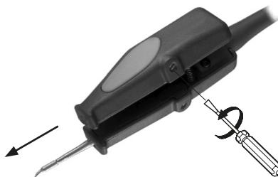
Loosen the screw and remove the cartridge.
