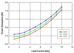
Fig. 3.3V.4: Power loss vs. load current and input voltage for Vout = 3.3V converter mounted vertically with air flowing from pin 10 to pin 1 at a rate of 200 LFM (1m/s) and Ta = 25°C.
