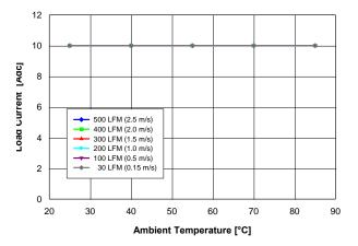
Fig. 2.5V.1: Available load current vs. ambient temperature and airflow rates for Vout = 2.5V converter mounted vertically with air flowing from pin 10 to pin 1, and maximum MOSFET temperature ≤ 120°C.
