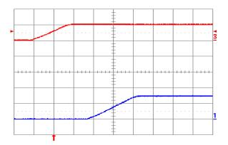
Fig. 1.5V.5: Turn-on transient for Vout = 1.5V with application of Vin at full rated load current (resistive) and 47μF external capacitance at Vin = 5V. Top trace: Vin (5V/div.); Bottom trace: output voltage (1V/div.); Time scale: 2ms/div.
