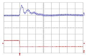
Fig. 3.3V.8: Output voltage response for Vout = 3.3V to negative load current step change from 5A to 2.5A with slew rate of -5A/μs at Vin = 5V. Top trace: output voltage (100mV/div.); Bottom trace: load current (5A/div.). Co = 100μF ceramic + 1μF ceramic. Time scale: 20μs/div.
