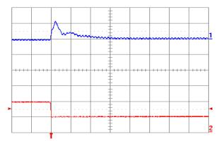
Fig. 1.0V.8: Output voltage response for Vout = 1.0V to negative load current step change from 5A to 2.5A with slew rate of -5A/μs at Vin = 5V. Top trace: output voltage (100mV/div.); Bottom trace: load current (5A/div.). Co = 100μF ceramic + 1μF ceramic. Time scale: 20μs/div.
