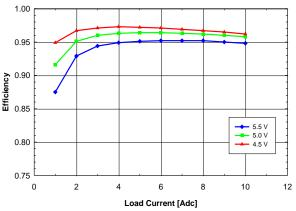
Fig. 3.3V.3: Efficiency vs. load current and input voltage for Vout = 3.3V converter mounted vertically with air flowing from pin 10 to pin 1 at a rate of 200 LFM (1m/s) and Ta = 25°C.
