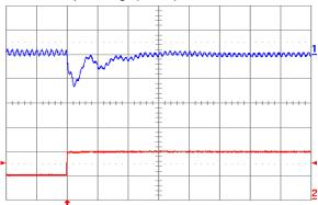
Fig. 2.5V.7: Output voltage response for Vout = 2.5V to positive load current step change from 2.5A to 5A with slew rate of 5A/μs at Vin = 5V. Top trace: output voltage (100mV/div.); Bottom trace: load current (5A/div.). Co = 100μF ceramic + 1μF ceramic. Time scale: 20μs/div.
