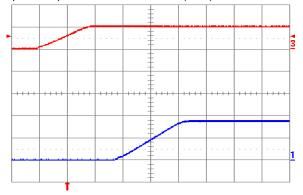
Fig. 1.8V.5: Turn-on transient for Vout = 1.8V with application of Vin at full rated load current (resistive) and 47μF external capacitance at Vin = 5V. Top trace: Vin (5V/div.); Bottom trace: output voltage (1V/div.); Time scale: 2ms/div.
