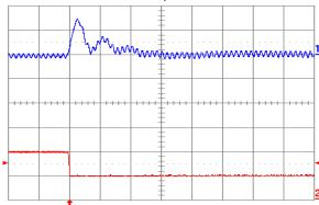
Fig. 2.5V.8: Output voltage response for Vout = 2.5V to negative load current step change from 5A to 2.5A with slew rate of -5A/μs at Vin = 5V. Top trace: output voltage (100mV/div.); Bottom trace: load current (5A/div.). Co = 100μF ceramic + 1μF ceramic. Time scale: 20μs/div.
