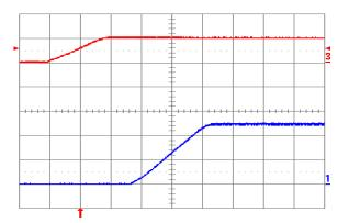
Fig. 2.5V.5: Turn-on transient for Vout = 2.5V with application of Vin at full rated load current (resistive) and 47μF external capacitance at Vin = 5V. Top trace: Vin (5V/div.); Bottom trace: output voltage (1V/div.); Time scale: 2ms/div.
