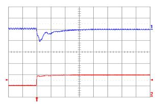
Fig. 0.7525V.7: Output voltage response for Vout = 0.7525V to positive load current step change from 2.5A to 5A with slew rate of 5A/μs at Vin = 5V. Top trace: output voltage (100mV/div.); Bottom trace: load current (5A/div.). Co = 100μF ceramic + 1μF ceramic. Time scale: 20μs/div.
