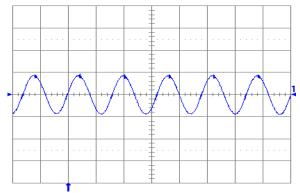
Fig. 3.3V.6: Output voltage ripple (20mV/div.) at full rated load current into a resistive load with external capacitance 47μF ceramic + 1μF ceramic and Vin = 5V for Vout = 3.3V. Time scale: 2μs/div.
