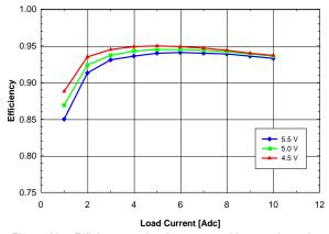
Fig. 2.5V.3: Efficiency vs. load current and input voltage for Vout = 2.5V converter mounted vertically with air flowing from pin 10 to pin 1 at a rate of 200 LFM (1m/s) and Ta = 25°C.
