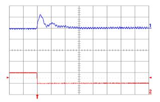
Fig. 1.5V.8: Output voltage response for Vout = 1.5V to negative load current step change from 5A to 2.5A with slew rate of -5A/μs at Vin = 5V. Top trace: output voltage (100mV/div.); Bottom trace: load current (5A/div.). Co = 100μF ceramic + 1μF ceramic. Time scale: 20μs/div.
