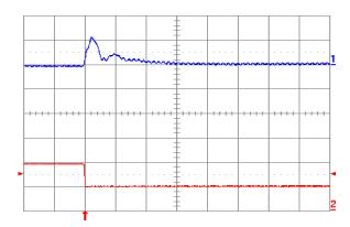
Fig. 0.7525V.8: Output voltage response for Vout = 0.7525V to negative load current step change from 5A to 2.5A with slew rate of -5A/μs at Vin = 5V. Top trace: output voltage (100mV/div.); Bottom trace: load current (5A/div.). Co = 100μF ceramic + 1μF ceramic. Time scale: 20μs/div.
