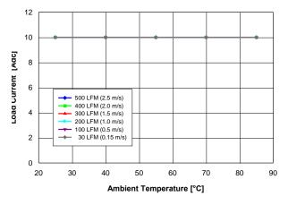
Fig. 2.0V.1: Available load current vs. ambient temperature and airflow rates for Vout = 2.0V converter mounted vertically with air flowing from pin 10 to pin 1, and maximum MOSFET temperature ≤ 120°C.
