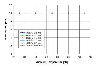
Fig. 1.8V.1: Available load current vs. ambient temperature and airflow rates for Vout = 1.8V converter mounted vertically with air flowing from pin 10 to pin 1, and maximum MOSFET temperature ≤ 120°C.
