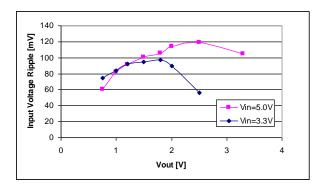
Fig. A: Input Voltage Ripple, CIN = 4x47 μF ceramic.
