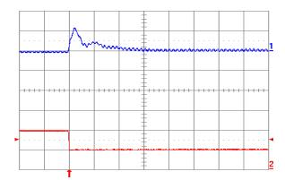
Fig. 1.2V.8: Output voltage response for Vout = 1.2V to negative load current step change from 5A to 2.5A with slew rate of -5A/μs at Vin = 5V. Top trace: output voltage (100mV/div.); Bottom trace: load current (5A/div.). Co = 100μF ceramic + 1μF ceramic. Time scale: 20μs/div.
