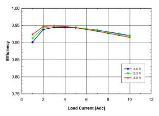
Fig. 1.8V.4: Efficiency vs. load current and input voltage for Vout = 1.8V converter mounted vertically with air flowing from pin 10 to pin 1 at a rate of 200 LFM (1m/s) and Ta = 25°C.
