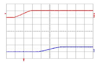
Fig. 0.7525V.5: Turn-on transient for Vout = 0.7525V with application of Vin at full rated load current (resistive) and 47μF external capacitance at Vin = 5V. Top trace: Vin (5V/div.); Bottom trace: output voltage (1V/div.); Time scale: 2ms/div.
