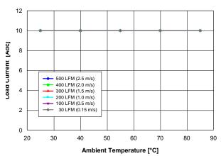
Fig. 0.7525V.1: Available load current vs. ambient temperature and airflow rates for Vout = 0.7525V converter mounted vertically with air flowing from pin 10 to pin 1, and maximum MOSFET temperature ≤ 120°C.
