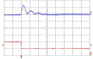
Fig. 2.0V.8: Output voltage response for Vout = 2.0V to negative load current step change from 5A to 2.5A with slew rate of -5A/μs at Vin = 5V. Top trace: output voltage (100mV/div.); Bottom trace: load current (5A/div.). Co = 100μF ceramic + 1μF ceramic. Time scale: 20μs/div.
