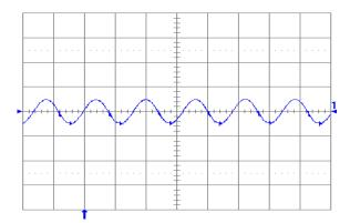
Fig. 1.0V.6: Output voltage ripple (20mV/div.) at full rated load current into a resistive load with external capacitance 47μF ceramic + 1μF ceramic and Vin = 5V for Vout = 1.0V. Time scale: 2μs/div.
