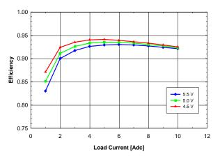
Fig. 2.0V.3: Efficiency vs. load current and input voltage for Vout = 2.0V converter mounted vertically with air flowing from pin 10 to pin 1 at a rate of 200 LFM (1m/s) and Ta = 25°C.
