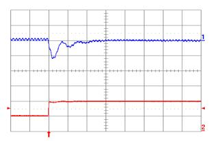
Fig. 1.5V.7: Output voltage response for Vout = 1.5V to positive load current step change from 2.5A to 5A with slew rate of 5A/μs at Vin = 5V. Top trace: output voltage (100mV/div.); Bottom trace: load current (5A/div.). Co = 100μF ceramic + 1μF ceramic. Time scale: 20μs/div.
