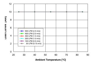
Fig. 2.0V.2: Available load current vs. ambient temperature and airflow rates for Vout = 2.0V converter mounted horizontally with air flowing from pin 10 to pin 1, and maximum MOSFET temperature ≤ 120°C.
