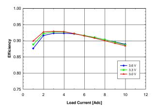
Fig. 1.2V.4: Efficiency vs. load current and input voltage for Vout = 1.2V converter mounted vertically with air flowing from pin 10 to pin 1 at a rate of 200 LFM (1m/s) and Ta = 25°C.
