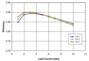
Fig. 0.7525V.4: Efficiency vs. load current and input voltage for Vout = 0.7525V converter mounted vertically with air flowing from pin 10 to pin 1 at a rate of 200 LFM (1m/s) and Ta = 25°C.
