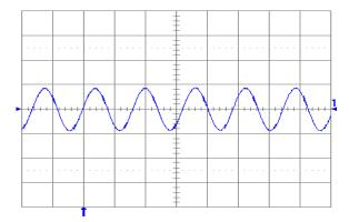
Fig. 2.0V.6: Output voltage ripple (20mV/div.) at full rated load current into a resistive load with external capacitance 47μF ceramic + 1μF ceramic and Vin = 5V for Vout = 2.0V. Time scale: 2μs/div.
