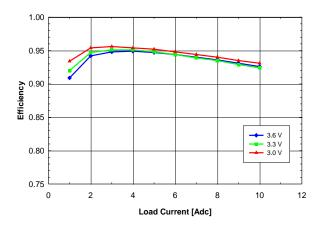
Fig. 2.0V.4: Efficiency vs. load current and input voltage for Vout = 2.0V converter mounted vertically with air flowing from pin 10 to pin 1 at a rate of 200 LFM (1m/s) and Ta = 25°C.
