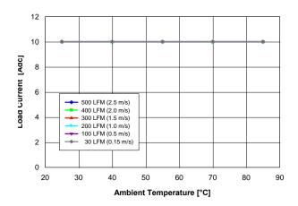
Fig. 1.2V.2: Available load current vs. ambient temperature and airflow rates for Vout = 1.2V converter mounted horizontally with air flowing from pin 10 to pin 1, and maximum MOSFET temperature ≤ 120°C.
