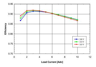
Fig. 1.0V.4: Efficiency vs. load current and input voltage for Vout = 1.0V converter mounted vertically with air flowing from pin 10 to pin 1 at a rate of 200 LFM (1m/s) and Ta = 25°C.
