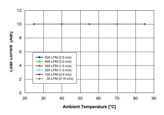
Fig. 1.0V.2: Available load current vs. ambient temperature and airflow rates for Vout = 1.0V converter mounted horizontally with air flowing from pin 10 to pin 1, and maximum MOSFET temperature ≤ 120°C.
