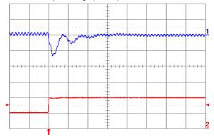
Fig. 2.0V.7: Output voltage response for Vout = 2.0V to positive load current step change from 2.5A to 5A with slew rate of 5A/μs at Vin = 5V. Top trace: output voltage (100mV/div.); Bottom trace: load current (5A/div.). Co = 100μF ceramic + 1μF ceramic. Time scale: 20μs/div.
