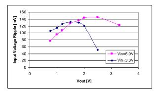
Fig. B: Input Voltage Ripple, CIN = 470 μF polymer + 2x47μF ceramic
