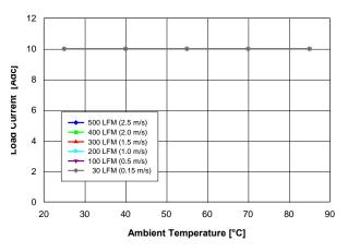
Fig. 1.5V.1: Available load current vs. ambient temperature and airflow rates for Vout = 1.5V converter mounted vertically with air flowing from pin 10 to pin 1, and maximum MOSFET temperature ≤ 120°C.
