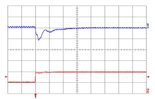
Fig. 1.0V.7: Output voltage response for Vout = 1.0V to positive load current step change from 2.5A to 5A with slew rate of 5A/μs at Vin = 5V. Top trace: output voltage (100mV/div.); Bottom trace: load current (5A/div.). Co = 100μF ceramic + 1μF ceramic. Time scale: 20μs/div.
