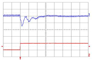
Fig. 3.3V.7: Output voltage response for Vout = 3.3V to positive load current step change from 2.5A to 5A with slew rate of 5A/μs at Vin = 5V. Top trace: output voltage (100mV/div.); Bottom trace: load current (5A/div.). Co = 100μF ceramic + 1μF ceramic. Time scale: 20μs/div.
