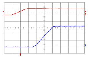
Fig. 3.3V.5: Turn-on transient for Vout = 3.3V with application of Vin at full rated load current (resistive) and 47μF external capacitance at Vin = 5V. Top trace: Vin (5V/div.); Bottom trace: output voltage (1V/div.); Time scale: 2ms/div.
