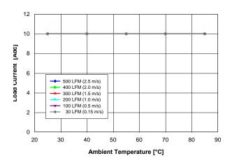
Fig. 1.8V.2: Available load current vs. ambient temperature and airflow rates for Vout = 1.8V converter mounted horizontally with air flowing from pin 10 to pin 1, and maximum MOSFET temperature ≤ 120°C.
