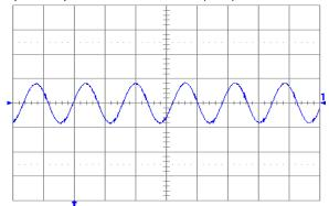
Fig. 1.8V.6: Output voltage ripple (20mV/div.) at full rated load current into a resistive load with external capacitance 47μF ceramic + 1μF ceramic and Vin = 5V for Vout = 1.8V. Time scale: 2μs/div.
