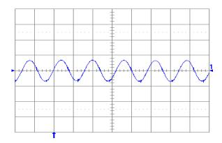
Fig. 1.5V.6: Output voltage ripple (20mV/div.) at full rated load current into a resistive load with external capacitance 47μF ceramic + 1μF ceramic and Vin = 5V for Vout = 1.5V. Time scale: 2μs/div.
