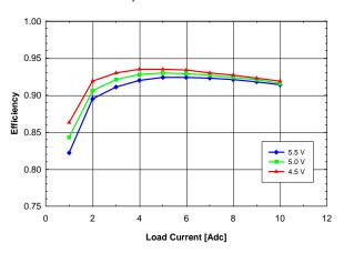
Fig. 1.8V.3: Efficiency vs. load current and input voltage for Vout = 1.8V converter mounted vertically with air flowing from pin 10 to pin 1 at a rate of 200 LFM (1m/s) and Ta = 25°C.
