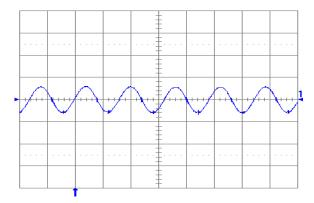
Fig. 1.2V.6: Output voltage ripple (20mV/div.) at full rated load current into a resistive load with external capacitance 47μF ceramic + 1μF ceramic and Vin = 5V for Vout = 1.2V. Time scale: 2μs/div.
