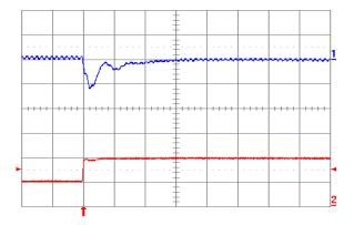
Fig. 1.2V.7: Output voltage response for Vout = 1.2V to positive load current step change from 2.5A to 5A with slew rate of 5A/μs at Vin = 5V. Top trace: output voltage (100mV/div.); Bottom trace: load current (5A/div.). Co = 100μF ceramic + 1μF ceramic. Time scale: 20μs/div.
