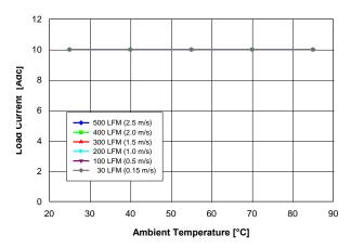
Fig. 1.5V.2: Available load current vs. ambient temperature and airflow rates for Vout = 1.5V converter mounted horizontally with air flowing from pin 10 to pin 1, and maximum MOSFET temperature ≤ 120°C.
