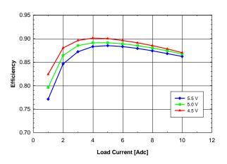
Fig. 1.0V.3: Efficiency vs. load current and input voltage for Vout = 1.0V converter mounted vertically with air flowing from pin 10 to pin 1 at a rate of 200 LFM (1m/s) and Ta = 25°C.
