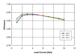
Fig. 1.5V.4: Efficiency vs. load current and input voltage for Vout = 1.5V converter mounted vertically with air flowing from pin 10 to pin 1 at a rate of 200 LFM (1m/s) and Ta = 25°C.
