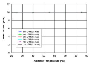
Fig. 2.5V.2: Available load current vs. ambient temperature and airflow rates for Vout = 2.5V converter mounted horizontally with air flowing from pin 10 to pin 1, and maximum MOSFET temperature ≤ 120°C.
