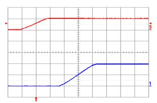
Fig. 2.0V.5: Turn-on transient for Vout = 2.0V with application of Vin at full rated load current (resistive) and 47μF external capacitance at Vin = 5V. Top trace: Vin (5V/div.); Bottom trace: output voltage (1V/div.); Time scale: 2ms/div.
