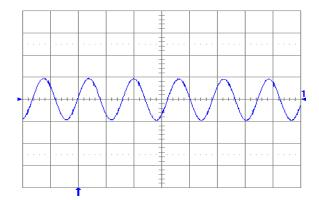
Fig. 2.5V.6: Output voltage ripple (20mV/div.) at full rated load current into a resistive load with external capacitance 47μF ceramic + 1μF ceramic and Vin = 5V for Vout = 2.5V. Time scale: 2μs/div.
