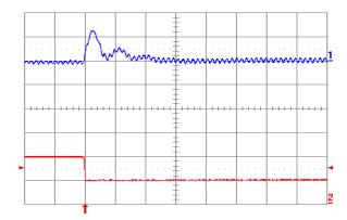
Fig. 1.8V.8: Output voltage response for Vout = 1.8V to negative load current step change from 5A to 2.5A with slew rate of -5A/μs at Vin = 5V. Top trace: output voltage (100mV/div.); Bottom trace: load current (5A/div.). Co = 100μF ceramic + 1μF ceramic. Time scale: 20μs/div.
