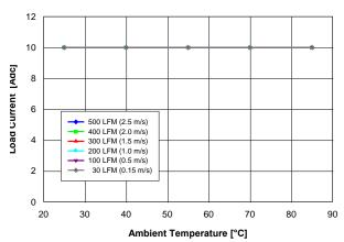
Fig. 0.7525V.2: Available load current vs. ambient temperature and airflow rates for Vout = 0.7525V converter mounted horizontally with air flowing from pin 10 to pin 1, and maximum MOSFET temperature ≤ 120°C.
