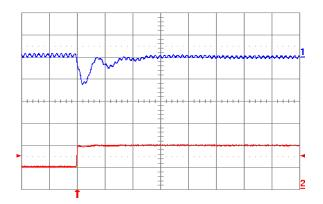
Fig. 1.8V.7: Output voltage response for Vout = 1.8V to positive load current step change from 2.5A to 5A with slew rate of 5A/μs at Vin = 5V. Top trace: output voltage (100mV/div.); Bottom trace: load current (5A/div.). Co = 100μF ceramic + 1μF ceramic. Time scale: 20μs/div.
