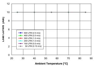
Fig. 3.3V.2: Available load current vs. ambient temperature and airflow rates for Vout = 3.3V converter mounted horizontally with Vin = 5V, air flowing from pin 10 to pin 1, and maximum MOSFET temperature ≤ 120°C.
