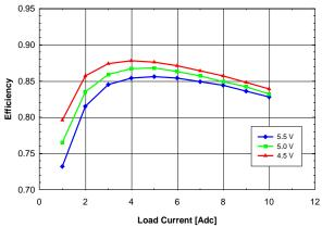
Fig. 0.7525V.3: Efficiency vs. load current and input voltage for Vout = 0.7525V converter mounted vertically with air flowing from pin 10 to pin 1 at a rate of 200 LFM (1m/s) and Ta = 25°C.
