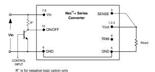
Fig. C: Circuit configuration for ON/OFF function.
