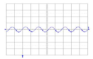
Fig. 0.7525V.6: Output voltage ripple (20mV/div.) at full rated load current into a resistive load with external capacitance 47μF ceramic + 1μF ceramic and Vin = 5V for Vout = 0.7525V. Time scale: 2μs/div.
