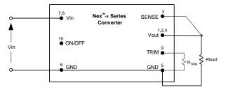
Fig. E: Configuration for programming output voltage.
